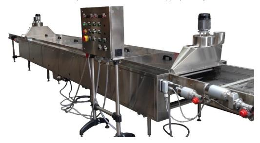
The number of distribution drawers determines the length of the kettle and therefore the hourly output.
