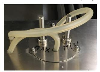
Possibility to adjust the height of the two water levels, minimum level (MIN) and maximum level (MAX).
