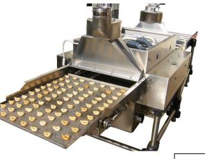
The regulation of the cooking time takes place with the adjustment of a knob placed in a separate and independent control panel.
